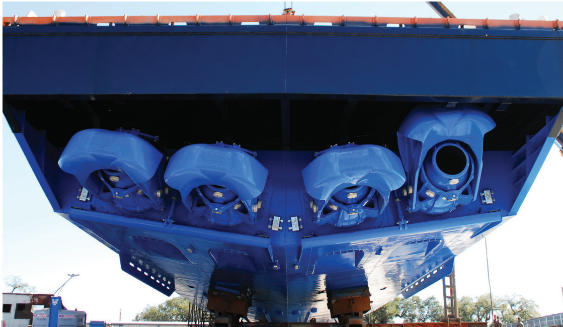
Above and Below: Crewboat "Aaron McCall" was the first vessel to be fitted with quadruple HamiltonJet HT900 waterjets
